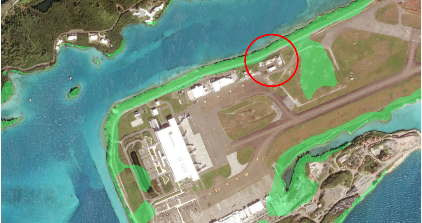
Figure 9.9 Sol Fuel Storage affected by saltwater inundation during the SSP5-8.5 100yr scenario
