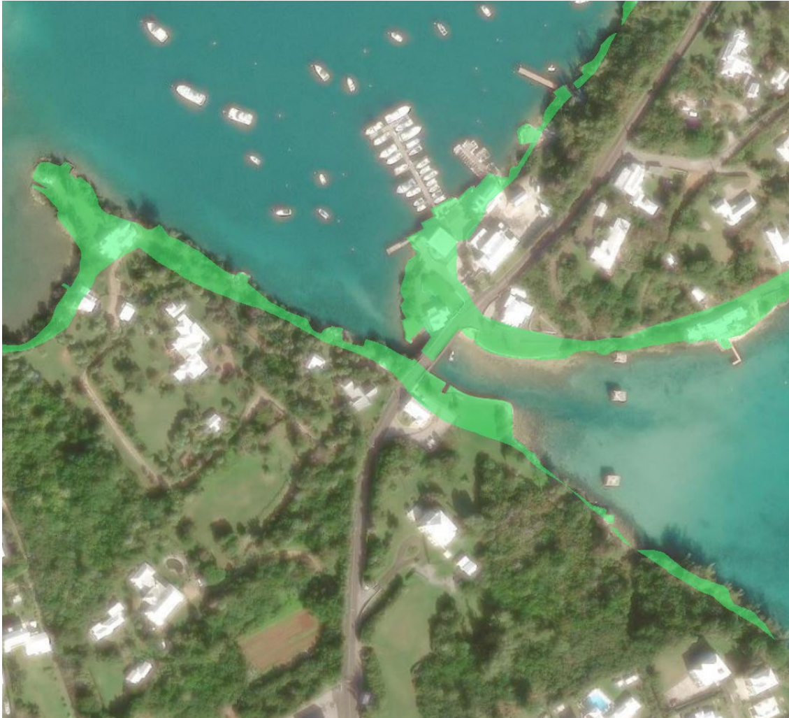
Figure 9.19 Somerset Bridge affected by saltwater inundation during the SSP5-8.5 100yr scenario (Note: data is not shown for suspended bridge deck sections)
