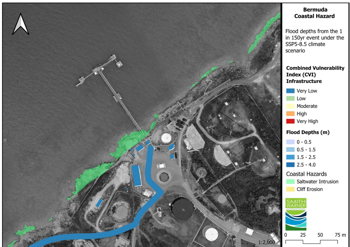
Figure 9.33 Flooding and Saltwater Intrusion along a small coastal strip around the Oil Docks Pier and surrounds (SSP5-8.5 100yr scenario)
