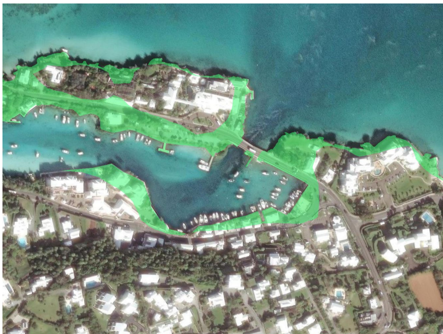
Figure 9.16 Flatts Bridge affected by saltwater inundation during the SSP5-8.5 100yr scenario (Note: data is not shown for suspended bridge deck sections)
