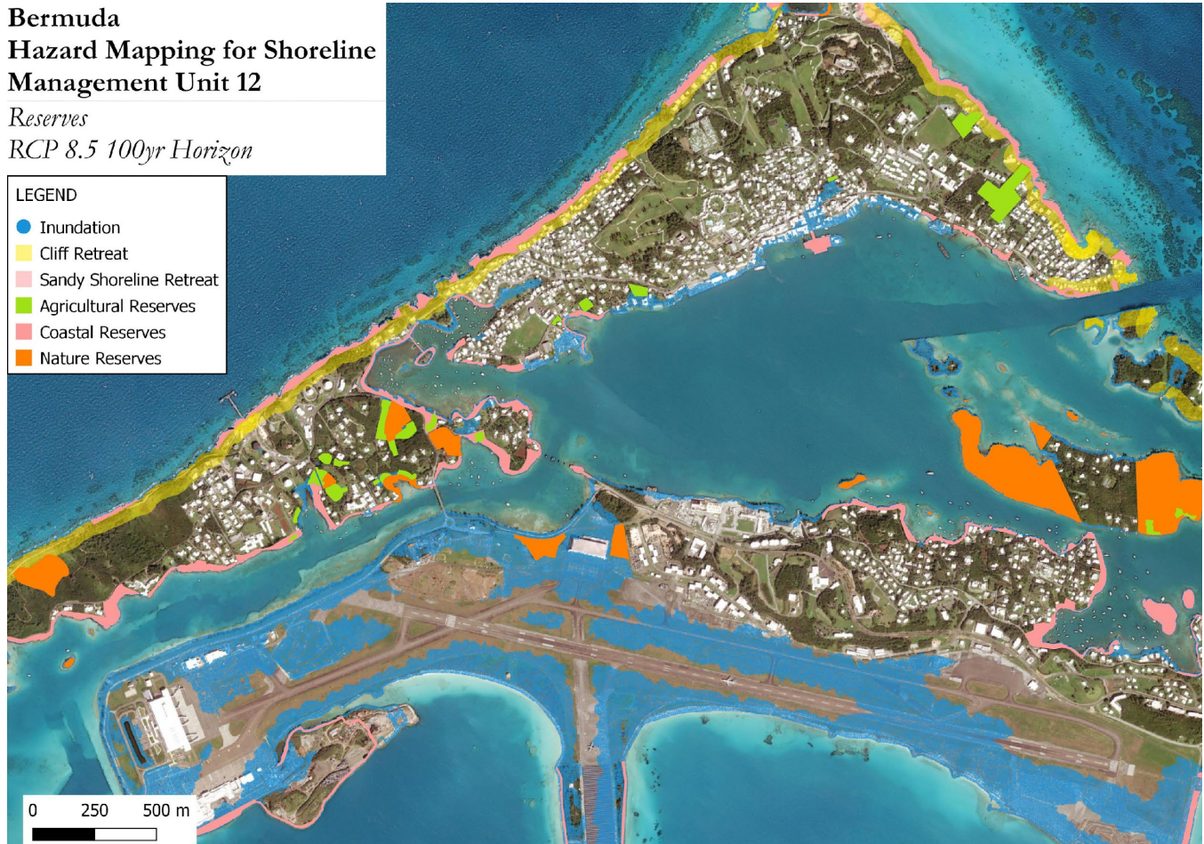
Figure 4.7 Impact of inundation and erosion from a RCP8.5, 100yr Horizon, 150yr event on Reserves within Management Unit 12
