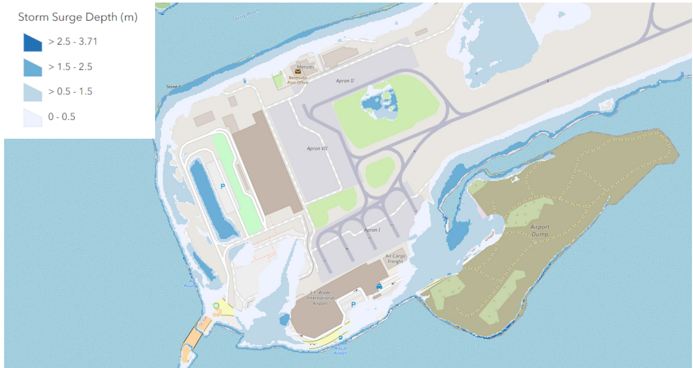
Figure 9.3 Airport terminal areas affected by flooding for the SSP5-8.5 100yr scenario
