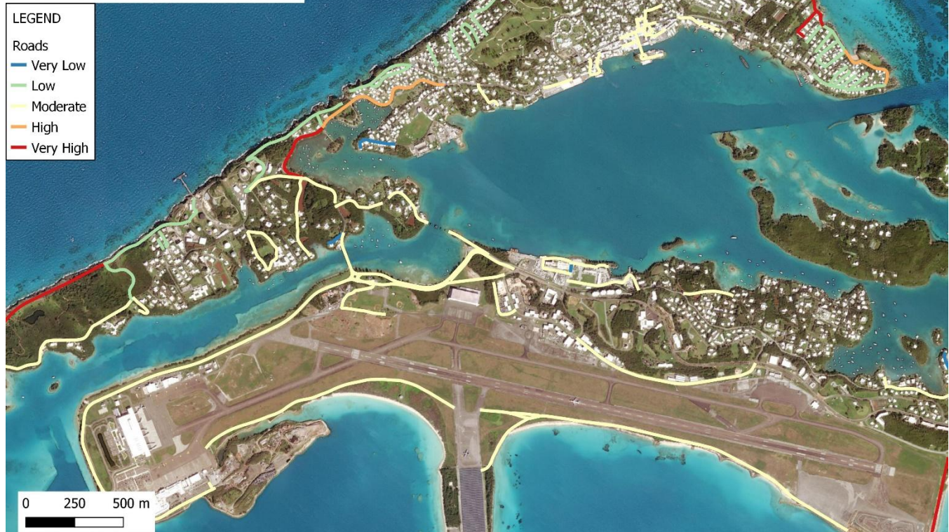
Figure 5.4 Road infrastructure vulnerability index for the RCP8.5, 100yr Horizon, 150yr event in SMU 12
