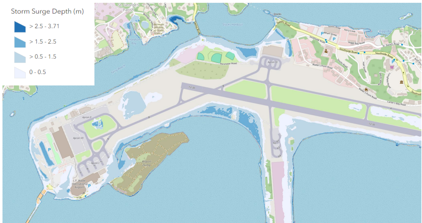
Figure 9.5 Airport perimeter roads affected by inundation during the SSP5-8.5 100yr scenario
