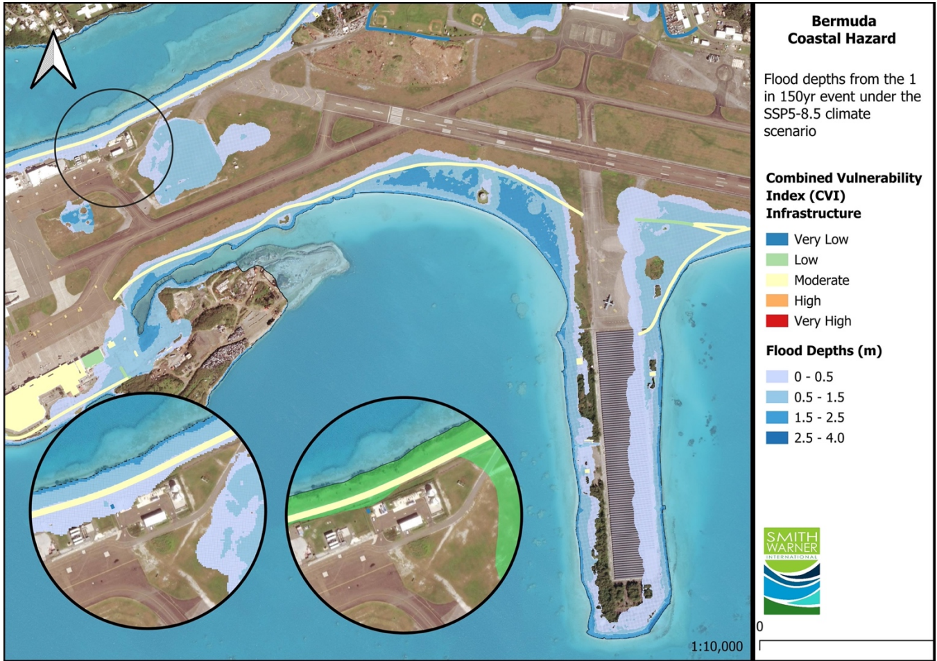
Figure 9.8 Sol Fuel Storage affected by inundation during the SSP5-8.5 100yr scenario
