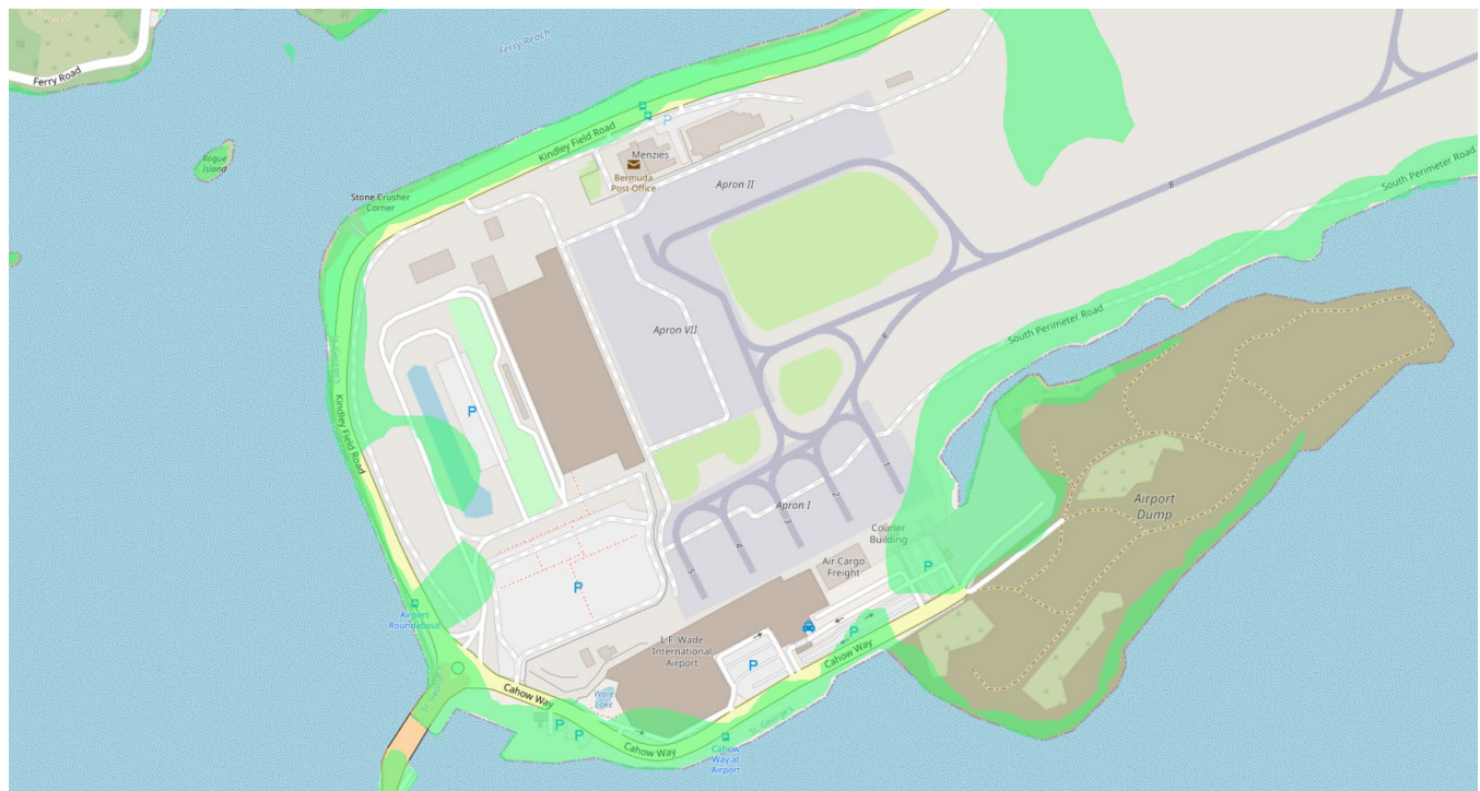
Figure 9.4 Airport terminal areas affected by saltwater intrusion for the SSP5-8.5 100yr scenario
