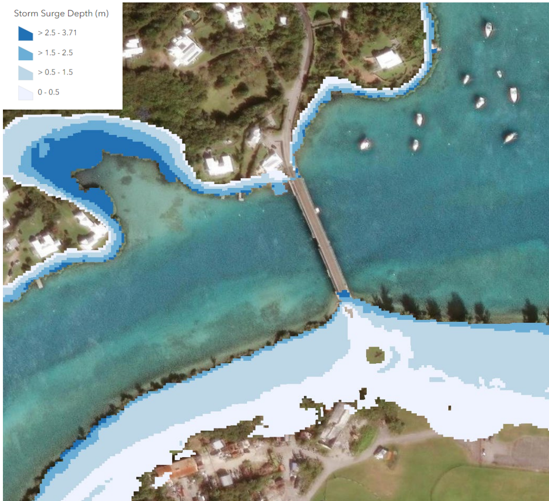
Figure 9.23 Swing Bridge affected by inundation during the SSP5-8.5 100yr scenario (Note: data is not shown for suspended bridge deck sections)
