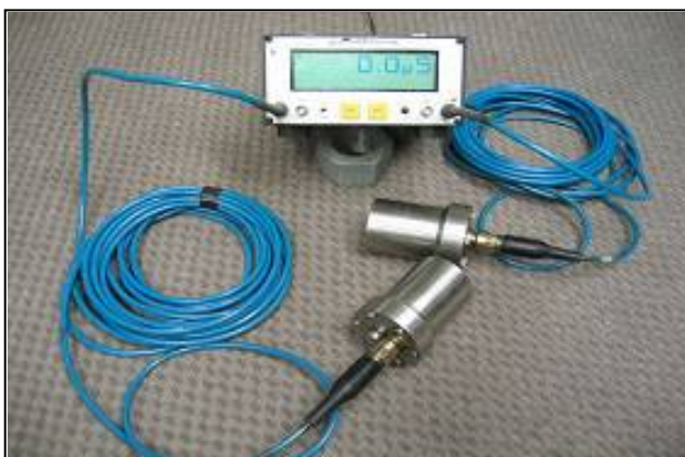
Figure 5-7 Ultrasonic Pulse Velocity Meter with Waterproof Cables and Transducers
