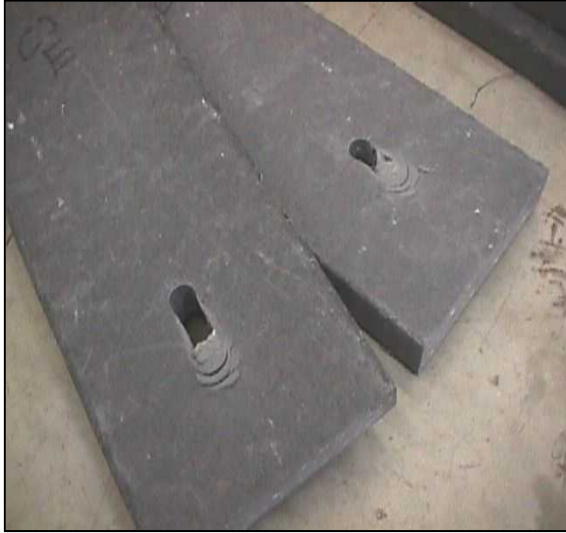
Figure 3-38 Yielding Around Hole of Composite Member
